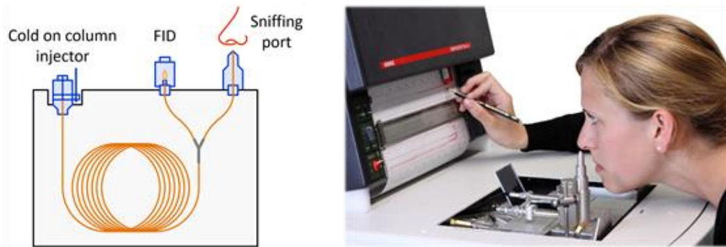
Figure 3: GC-O, basic principle (left) and application (right) (illustration: Martin Steinhaus)
