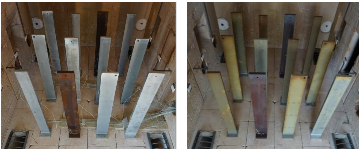
Figure 61: Setup of the second fire test before (left) and after (right) the thermal impact
