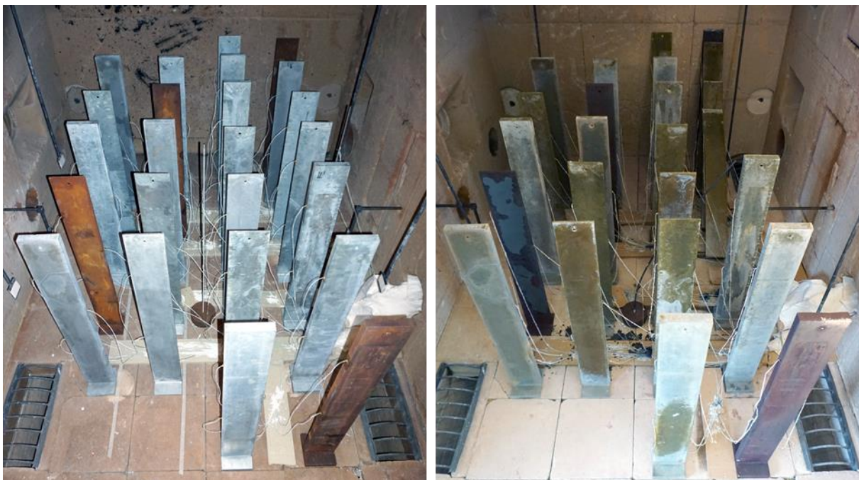
Figure 53: Setup of the first fire test before (left) and after (right) the thermal exposure
