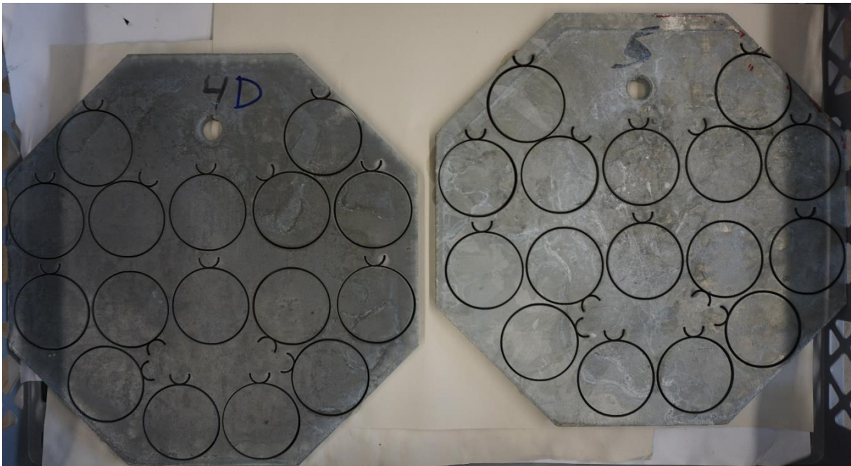
Figure 94: Carrier plates after water jetting with the corresponding test samples
