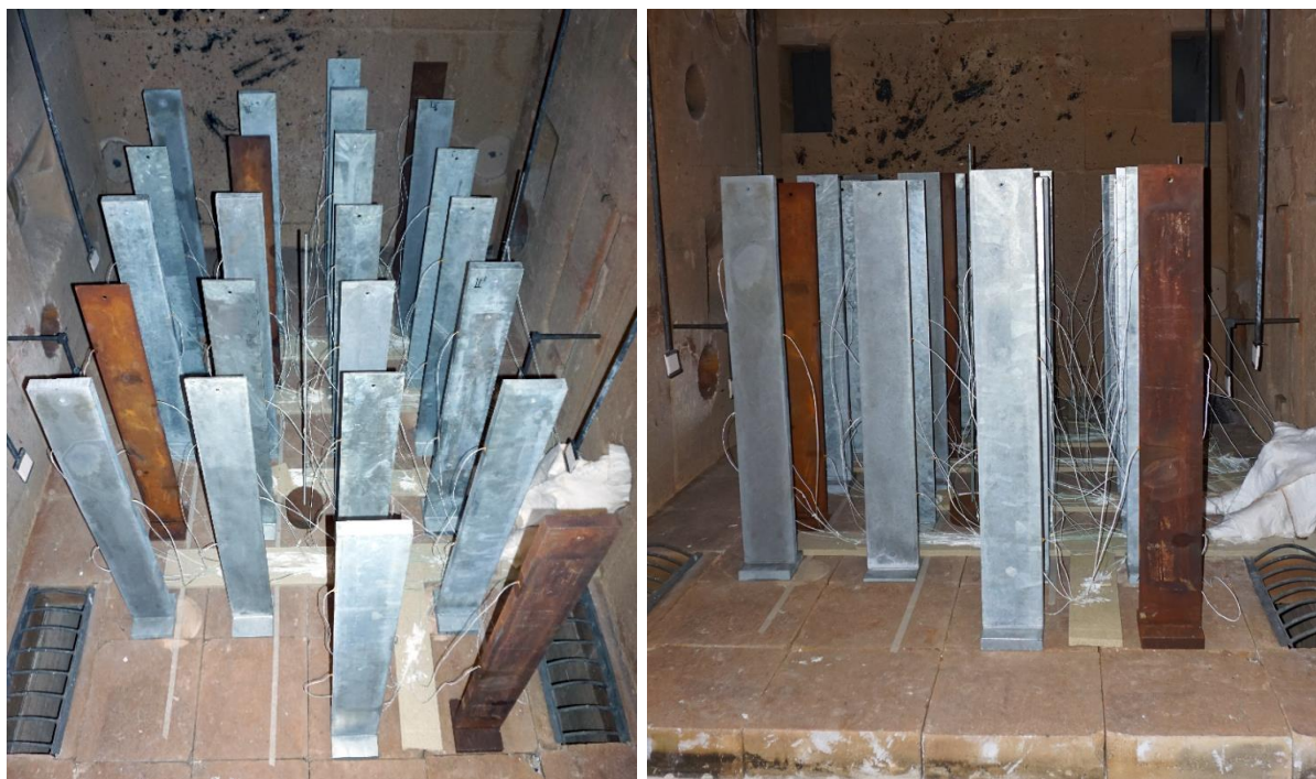
Figure 19: Setup of the first full fire test
