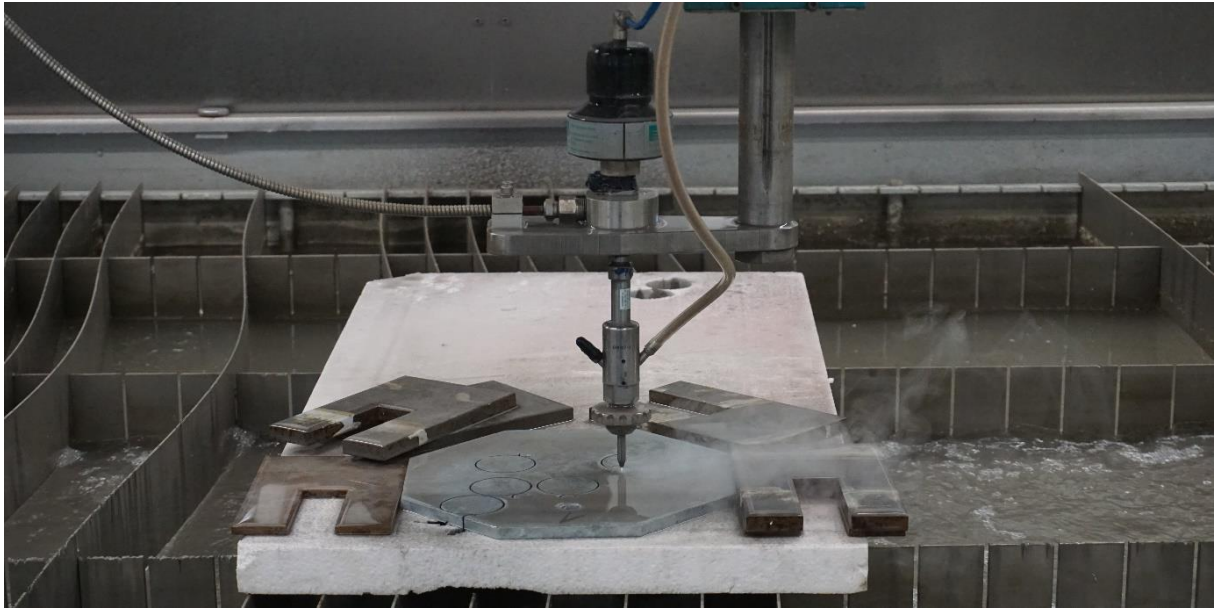
Figure 93: Preparation of the test samples ( d = 50 mm) out of the octagon carrier plate by water jetting
