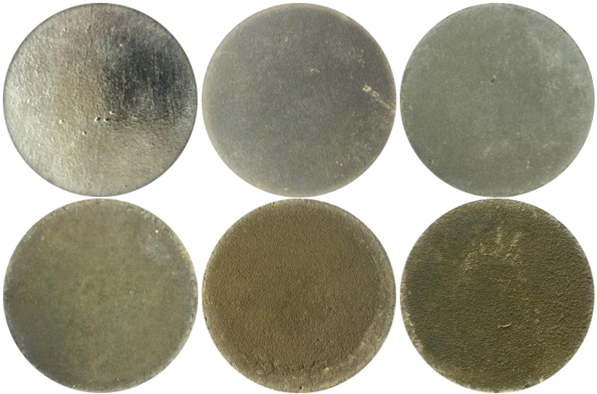
Figure 79: Samples of the same carrier plate of category A ('3N'), which have been affected by different temperature stages. From left to right: 1. Row: Original sample (20 °C); after 497 °C and 564 °C; 2. Row: after 693 °C, 808 °C and 846 °C
