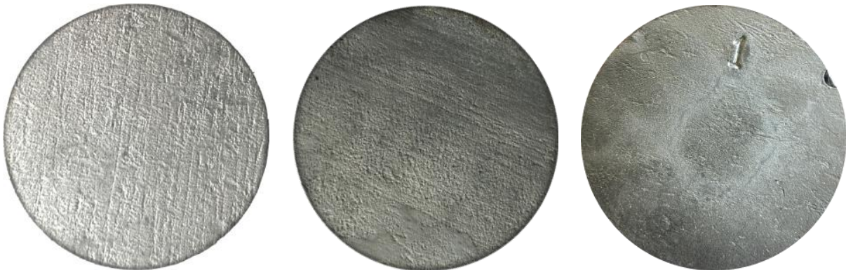
Figure 35: Specimen of category B: Stored inside (left); stored outside (middle); specimen of CTU, stored inside (right)
