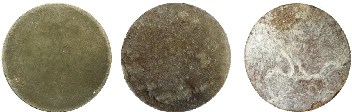
Figure 32: Same specimen of category A as in Figure 31 after the thermal exposure of the EP-T: Newly HDG after 714 °C (left); two samples with respective adverse initial storage: afterwards stored 'inside' (middle) and afterwards stored 'outside' (right) each after 850 °C
