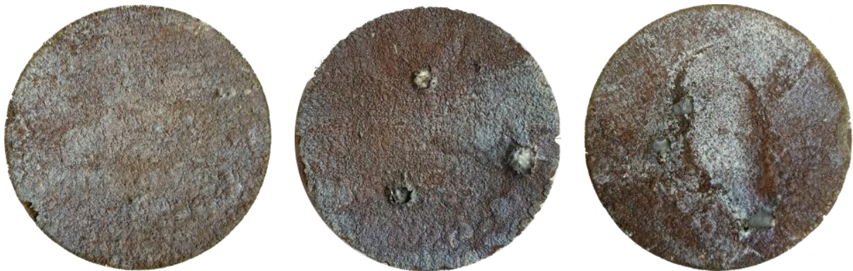
Figure 40: Same specimen of category D as in Figure 39 after the thermal impact of the EP-T: samples with respective adverse initial storage after 800 °C (left) and 850 °C (middle & right)
