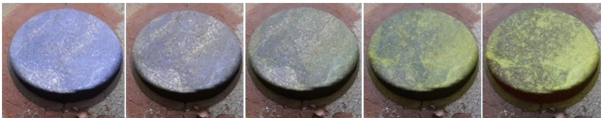
Figure 87: Thermochromism during heating of a hot-dip galvanized sample. From left to right: 22 °C, 340 °C, 510 °C, 650 °C, 810 °C
