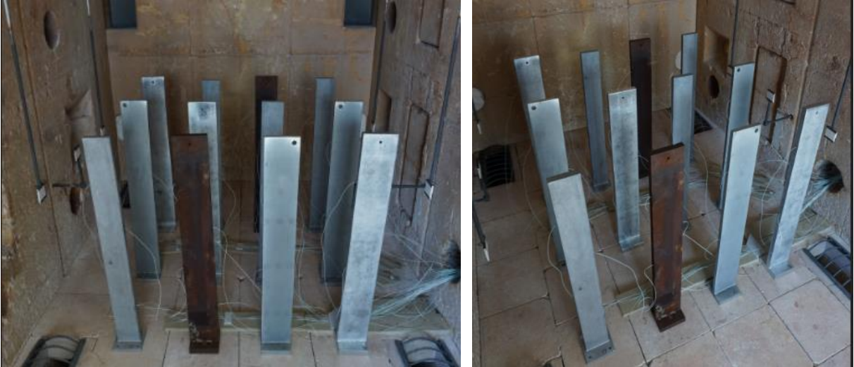
Figure 22: Setup of the second full fire test
