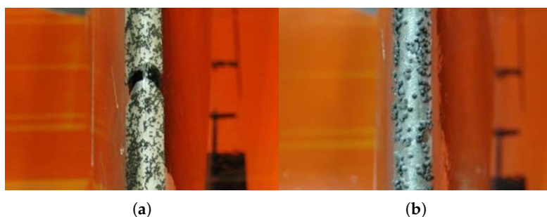
Figure 4. Additional very rough carborundum grits. (a) h_d/l_\mu = 0.125\% ( h_d = 1 mm); (b) h_d/l_\mu = 0.250\% ( h_d = 2 mm).
