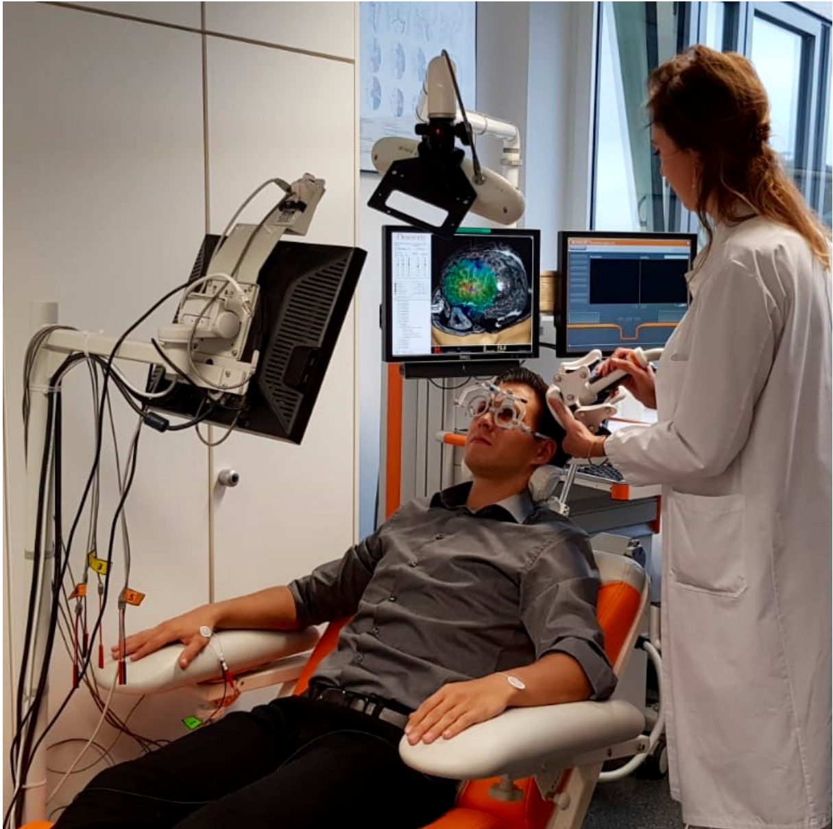
Fig. 5: Setup of the Nexstim eXimia system with stereotactic camera, stimulation coil, video screen for task pictures, video camera, and two further screens for navigation control and task adjustments.
