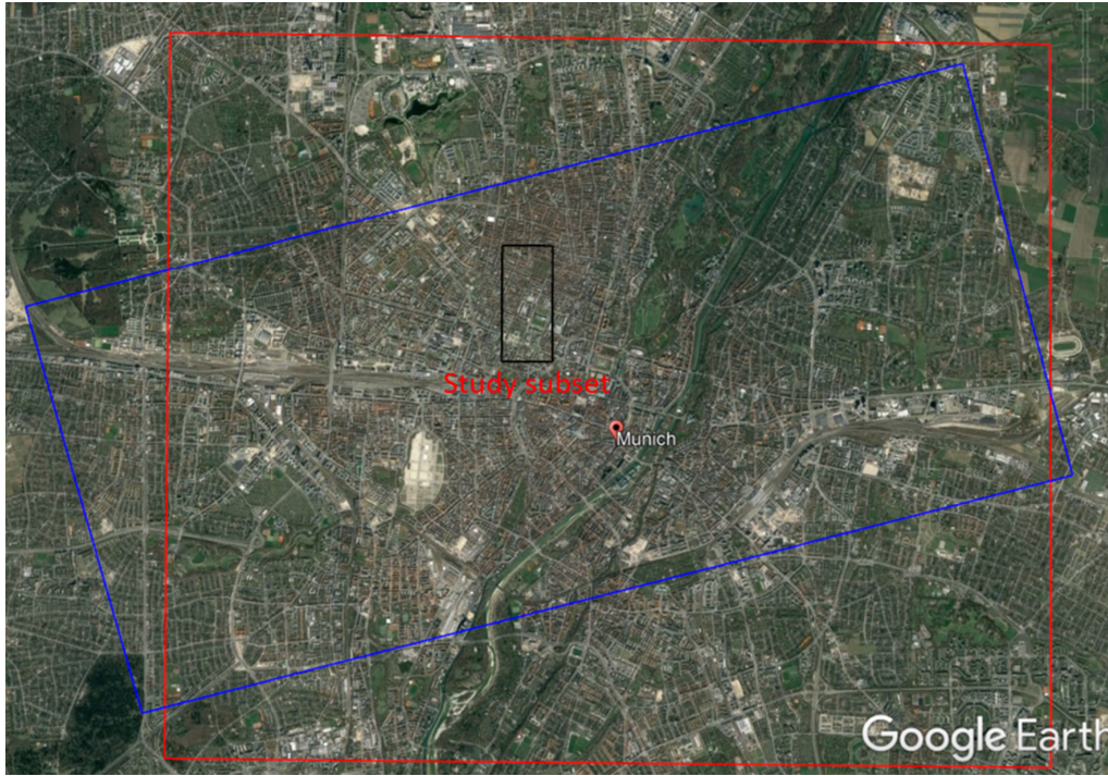
Fig. 5. Display the location of SAR-optical image pairs of the Munich study area. The red and blue rectangles identify areas covered by the WorldView-2 and TerraSAR-X images, respectively, and the black rectangle displays the study subset selected for stereogrammetric 3D reconstruction over Munich. (For interpretation of the references to color in this figure legend, the reader is referred to the web version of this article.)
