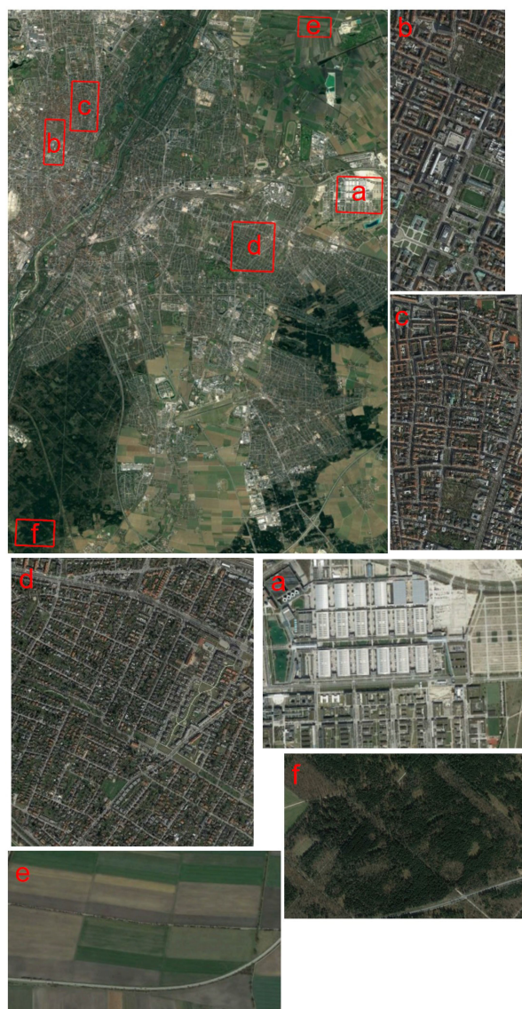
Fig. 3. Display of the study subsets selected from different urban land types for TanDEM-X raw DEM fusion over Munich city. a) Industrial area ( 1.5 \text{ km} \times 1.2 \text{ km} ). b) Inner city 1 ( 1.5 \text{ km} \times 0.6 \text{ km} ). c) Inner city 2 ( 1.6 \text{ km} \times 0.9 \text{ km} ). d) Residential area ( 1.6 \text{ km} \times 1.3 \text{ km} ). e) Agricultural ( 1.05 \text{ km} \times 0.6 \text{ km} ). f) Forested ( 1.25 \text{ km} \times 0.85 \text{ km} ).
