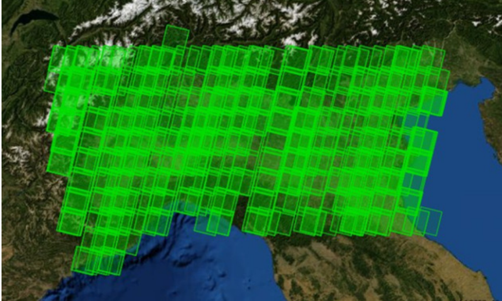
Figure 2.5: Stack of stereo Cartosat-1 images acquired over the north of Italy for producing a DEM on a large scale [68]
