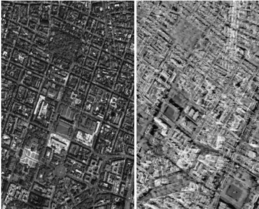
Fig. 7. Display of SAR-optical sub-scenes extracted from Munich study areas (the left-hand image is from WorldView-2, right-hand image is from TerraSAR-X).
