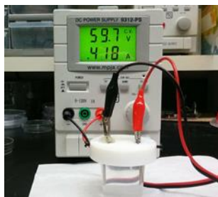
Figure 2.2-1. Experimental setup of TiO 2 nanotube array anodization, with two Ti-foils used as anode and cathode with benchtop power supply (DC MPJA POWER SUPPLY 9312-PS) for anodization at 60 V in an electrolyte containing 97:3 v/v ethylene glycol and deionized water (0.03 wt.-% NH 4 F).
