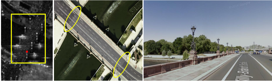
Figure 5.14: (Left) The TerraSAR-X test image of one bridge area in Berlin as cropped by the yellow rectangle. The red point is the reference point for the elevation and seasonal motion reconstruction in this area. (Middle) The associated orthorectified optical image, generated using semi-global matching [Hir08]. (Right) The streetview image from Google StreetView.
