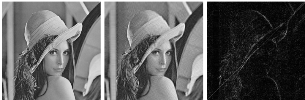
Figure 5.2: (Left) Original image. (Middle) Reconstructed image based on 50 singular values. (Right) The residuals. By reconstructing the image based on only 50 singular values, it can be observed in Figure 5.2 that the main information can be preserved.
