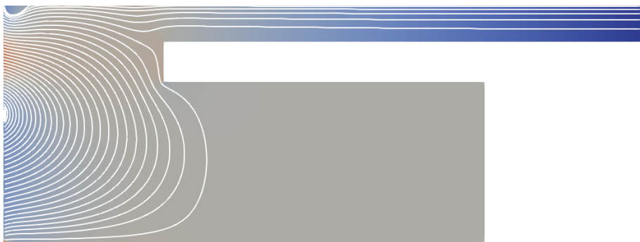
Figure 8.7.: Streamlines of the optimal flow
