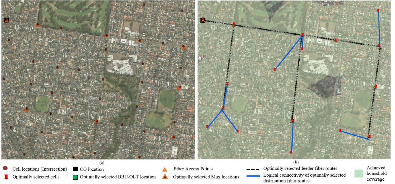
Fig. 2. (a) Input dataset; (b) Optimal solution of 10 DWDM-PON 1:8 split x-haul network and 99% household coverage with 25Mbps capacity requirement.
