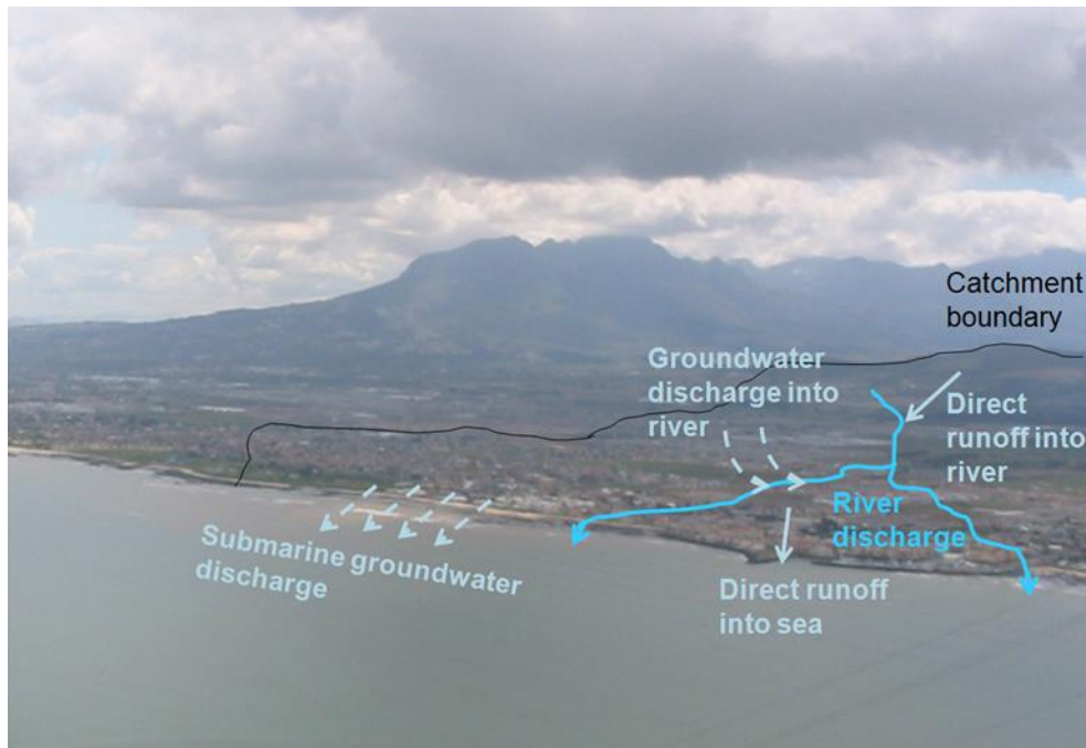
Figure 1: Representation of submarine groundwater discharge in a catchment
