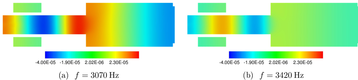
Figure 8.26: Acoustic density distribution \Re\{\hat{\rho}\} , [kg/(m 3 )] for the 3D model at the eigenfrequencies, based on the LES mean flow field.
