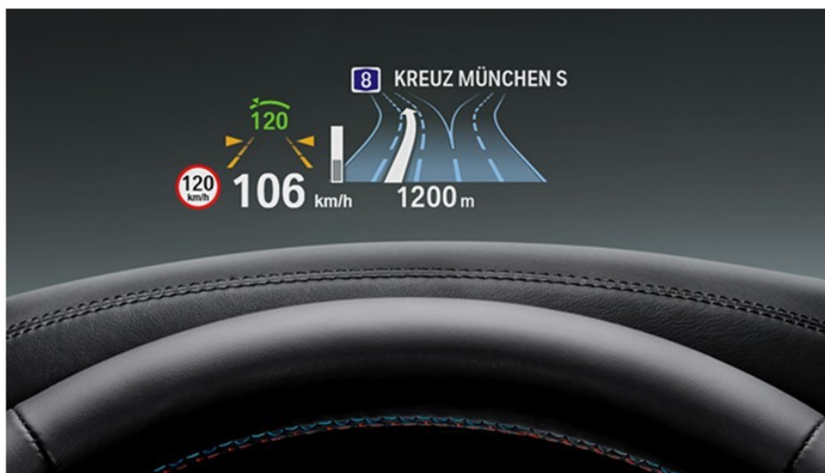
Figure 3.6.: Example of a windshield HUD showing speed information, speed limit, lane departure warning as well as navigational information. (Courtesy of BMW)
