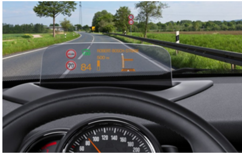
Figure 3.8.: Example of a combiner HUD showing speed information, speed limit, road sign as well as navigational information. (Courtesy of Bosch)
