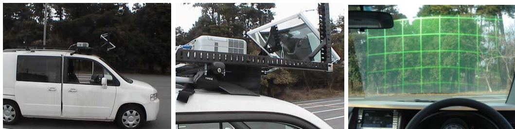
Figure 3.9.: Prototypical implementation of a large FoV HUD enabling AR visualisations. [SKKO06]
