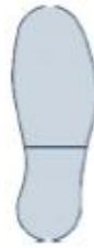
Figure 1. Detecting area division of the fore and rear foot part in loadsol force insole (adapted from [36]).
