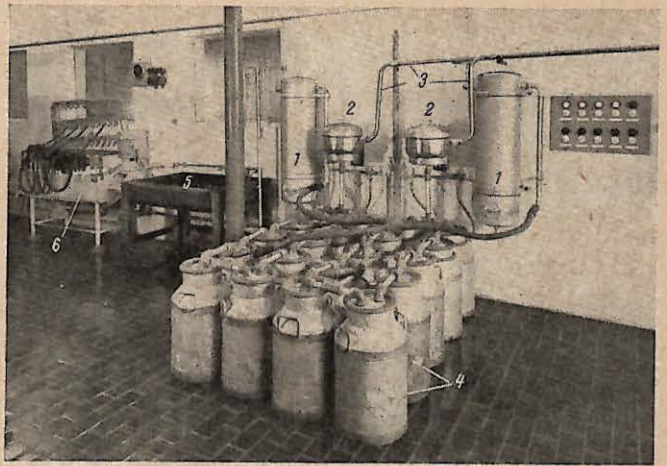
5) Storage, cleaning, and cooling room forming a part of a "Westfalia" machine milking stand equipped with a "Favorit" washer for cleaning milk cans and milker units by Ernst Göbel KG.
