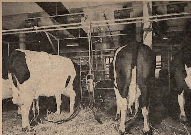
2) "Westfalia" filter-type milking system (Westfalia Separator AG.) 1 double filter-type milking unit for milking two cows at a time similar to the two-pail milking system), 2 vacuum hose to pulsator, 3 milk hose serving both milkers, 4 vacuum line, 5 milk line
