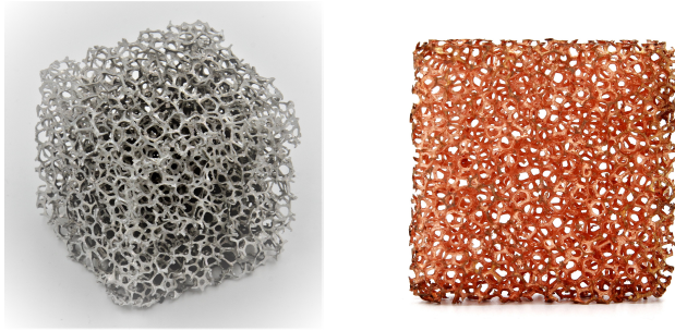
Figure 3.8: Pictures of a metallic foam with an irregular structure. Samples provided by Marie-Line Zanota, LGPC Lyon. Photos taken by Tobias Scheuermann, TUM Garching.
