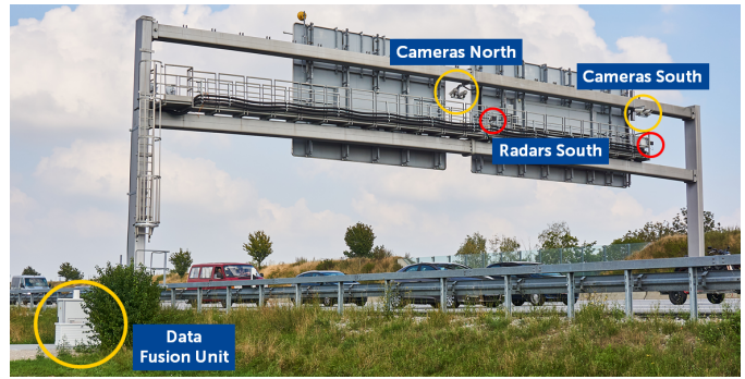
Fig. 1: One of our measurement points on the highway A9. All sensor information is processed by the local Data Fusion Unit. The two radars directed towards north are installed on the other side of the gantry bridge and hence not visible from this perspective.
