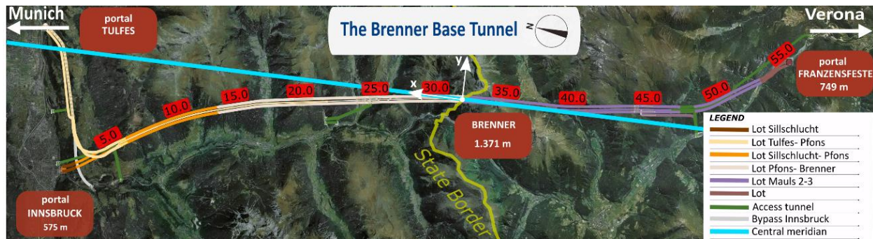
Figure 1. Plan of the BBT project's site with topography, the state border Austria-Italy and the tunnels. Central meridian, project's origin, and coordinate axes are also marked (Markič et al 2019).
