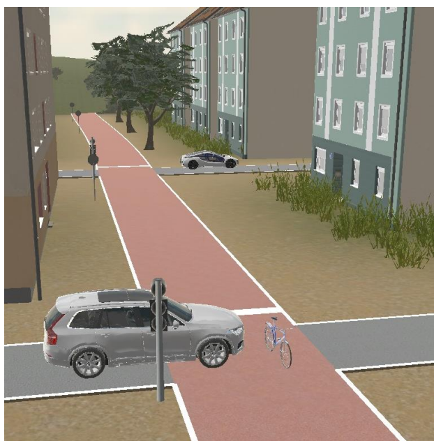
Figure 11. Testing the interactions between bicyclists and vehicle drivers by varying the sight distances of the vehicle drivers in the simulated VR environment.
