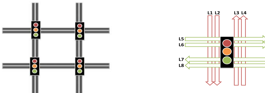
(a) Road network. Each road has 4 lanes(2 in each direction), a fixed Length_Y = 900m and a maximum speed v_Y^{max} with different values(for each scenario).
