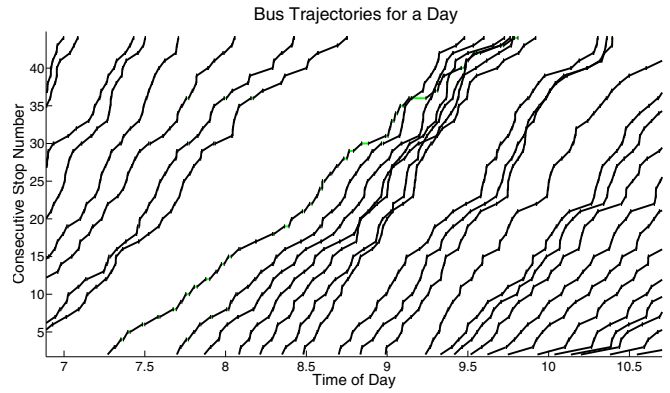
Fig. 3. Bus trajectories produced by the simulation during morning rush hour. The green horizontal lines indicate boarding of passengers on the stops. The phenomenon of bus bunching can be clearly observed resulting in larger periods of time where no buses are available for the passengers.
