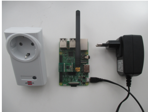
Figure 4.16: Possible charge delay implementation using remote-controlled switches
