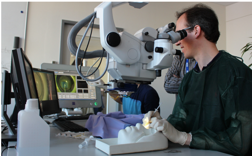
Fig. 3.3. Surgeon performing DALK on an ex vivo porcine eye using the proposed VR solution. With the virtual representation of the procedure, the surgeon can perform the surgery without looking at the real scene.
