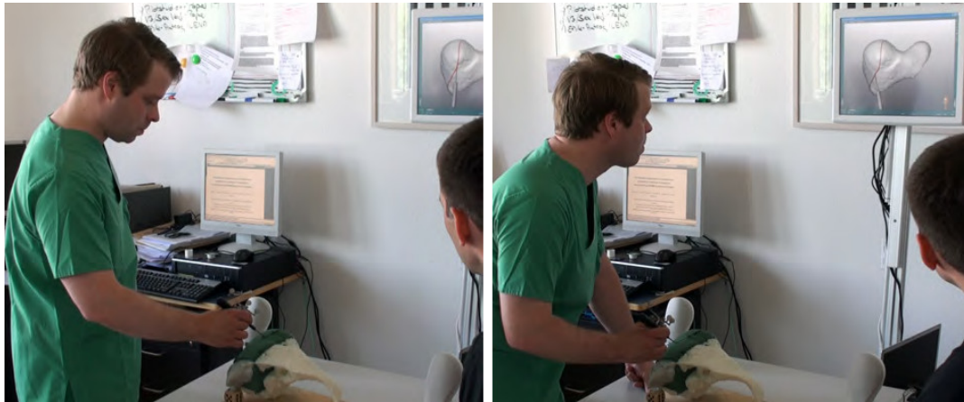
Fig. 2.3. Simulated liver surgery with auditory feedback. The participating surgeon uses the tracked instrument to mark the planned resection line on the liver phantom. The surgeon mostly observes the liver phantom when auditory feedback is available (left) and repeatedly glances at the navigation system screen when no audio feedback is present (right).
