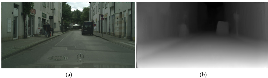
Figure 7. Disparity map obtained from a single image using monodepth [25]. (a) Original image. (b) Disparity map.
