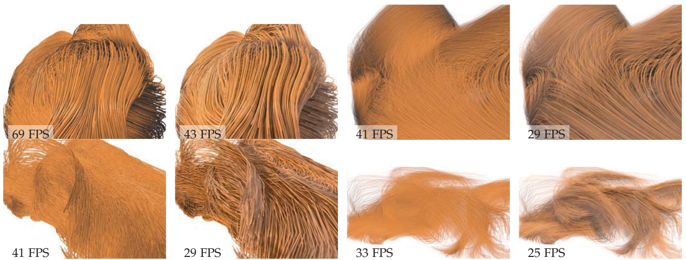
Fig. 19: Lines are rendered with local illumination (left) and soft shadows in combination with ambient occlusions (right). When rendering huge amounts of semi-transparent curves, single curves cannot be distinguished any longer. Ambient occlusions help to distinguish individual curves, since less light is reaching occluded curves. Shadow effects enhance the overall structure of the dataset and indicate the relative position of curves to each other. In combination with ambient occlusions, details in shadowed regions are preserved.
