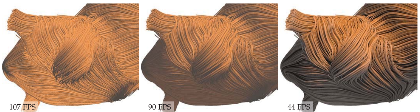
Fig. 20: First: Local illumination. Second: Soft shadows from line density values via cone-tracing. Third: Soft shadows in combination with ambient occlusion using 50 sample rays per voxel. The Aneurysm II dataset is shown, while continuously updating corresponding illumination values.
