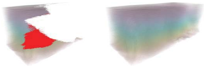
Fig. 17: Left: GPU rasterization using fragment linked lists fails due to memory limitations. Red indicates 512 or more fragments fall onto a pixel, when not all fragments could be stored due to memory limitations the pixel is set to white. Right: Voxel-based ray-casting renders at 23 ms.
