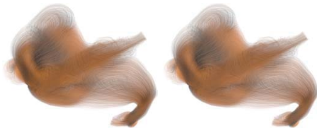
Fig. 11: Left: Transparency rendering using fragment linked lists on the GPU (160 ms, 600 MB fragment list). Right: GPU ray-casting (24 ms, 256^3 voxel grid, curve-face intersections quantized to 16^2 bins, 60 MB voxel representation).
