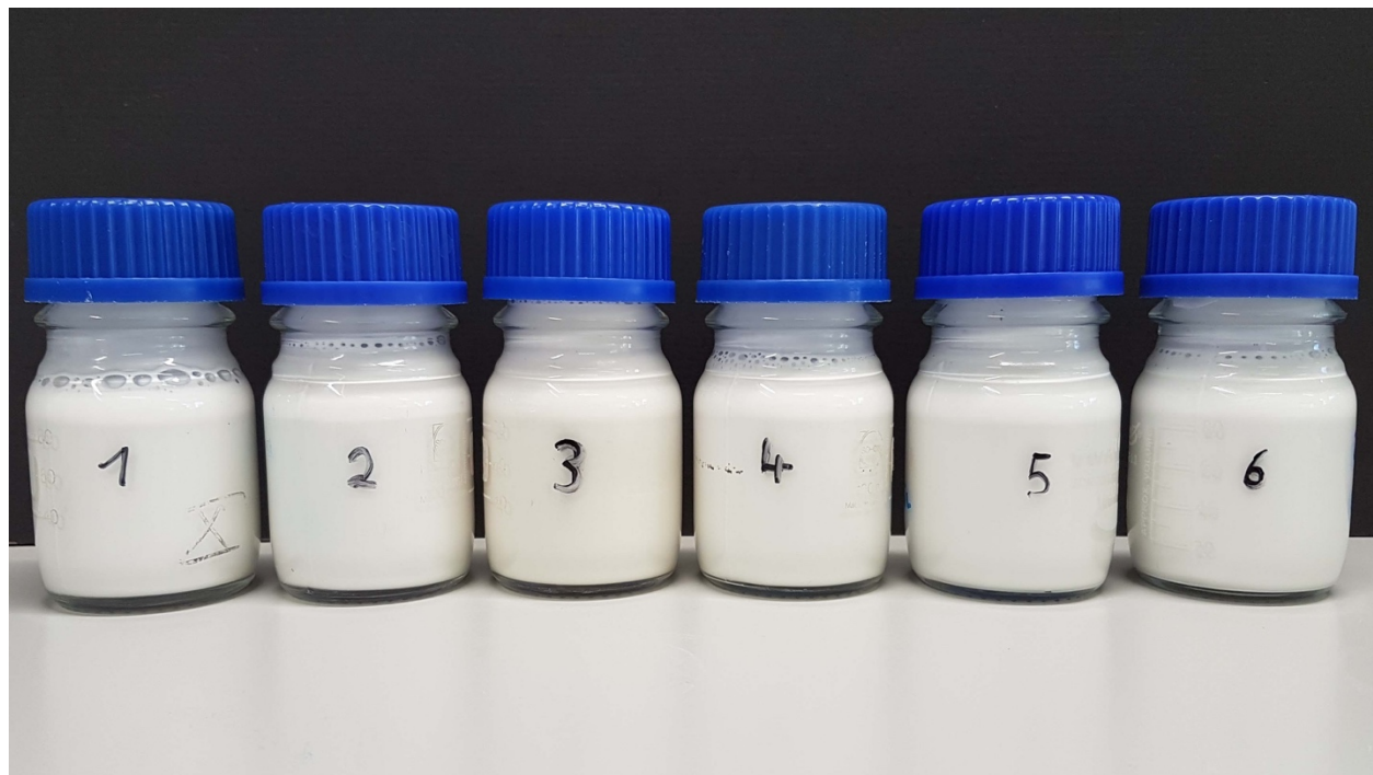
Figure 51: Visual inspection of O/W emulsions with protein type and content stored at 4 °C for 9 d after manual agitation. After storage at 4 °C for 9 d (see Figure 50B) O/W emulsions agitated manually by gently inverting the flask and afterwards reevaluated for inspected visually for phase distribution. Emulsions are numbered according to the protein type and concentration in the aqueous phase. Numbers in brackets (#) refer to the number coding in Tables 21 and 22: 1: 0 % protein (#17) 2: 2.5 % peptone (#18); 3: 10 % peptone (#19); 4: 2.5 % WPI (#20); 5: 10 % WPI (#21); 6: 2.5 % casein (#22).
