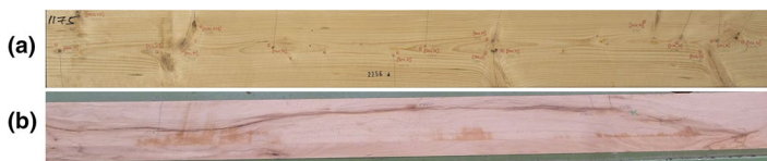
Fig. 1 Fiber deviations in softwoods and hardwoods. a Spruce board, b beech board
