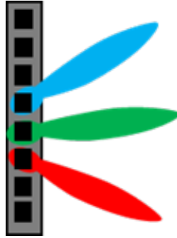
Figure 2.11.: Elevation beamforming from a vertical ULA
