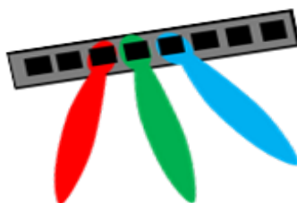
Figure 2.10.: Azimuth beamforming from a horizontal ULA
