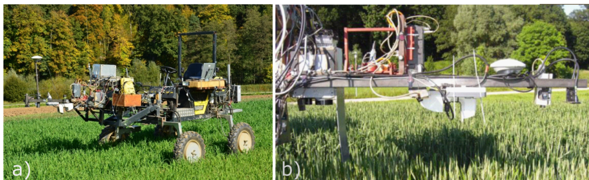
Figure 5: Mobile sensor platform Phenotrac 4 (a) and sensor carrier arm attached to the front of the sensor platform (b). The aperture of the hyperspectral sensor is positioned on the right side and connected with the actual sensor (silvery box in the left image) via optical fibers.
