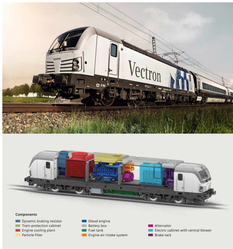
Figure 7.3: Siemens Train - Vectron and its structural components [119].
