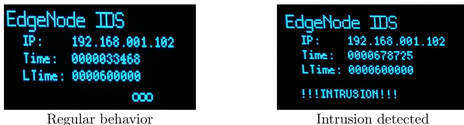
Figure 4.10: Current state of the IDS on the edge node display.
