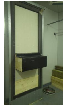
Figure 5: Hygrothermal test cells and wall-balcony sample (exterior view)
