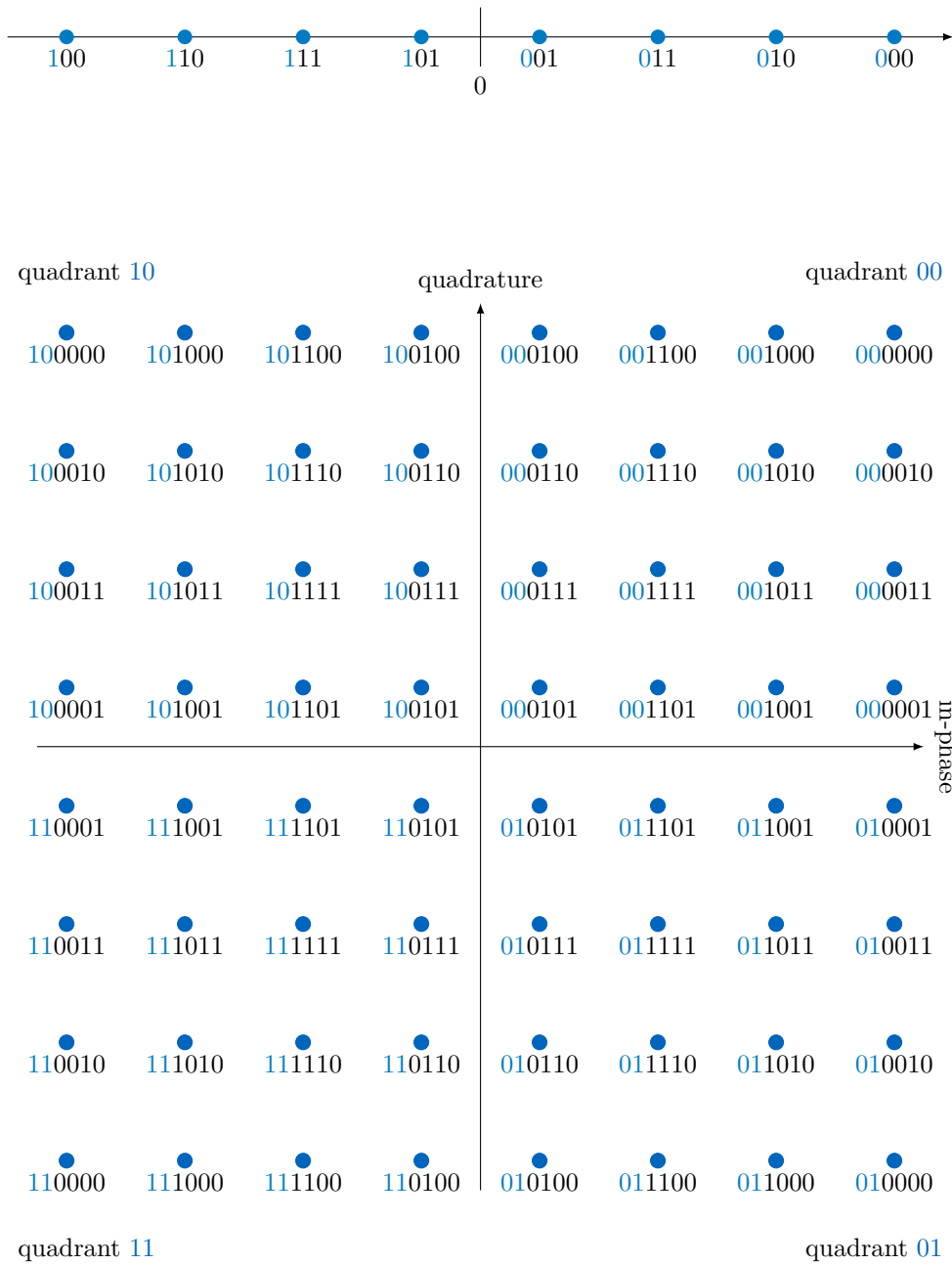
Figure 2.10: 8-ASK and 64-QAM constellations with BRGC labelings.
