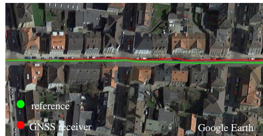
Fig. 4. Low GNSS measurement quality due to local effects [cf. 5, 6].
