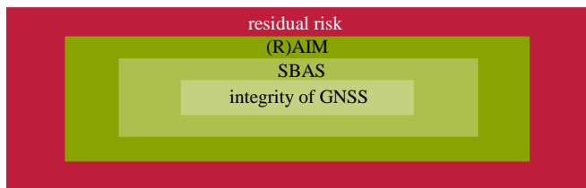
Fig. 18. Integrity layers of GNSS-based localization [cf. 5].
