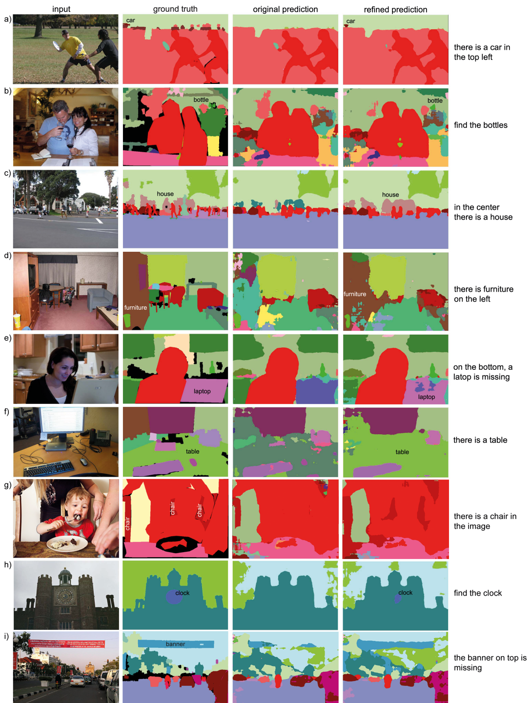
Figure 8.4 Qualitative results using find hints. The guided network is able to recover from ambiguities and difficult cases, such as heavily occluded objects, and also refine partially predicted segments.
