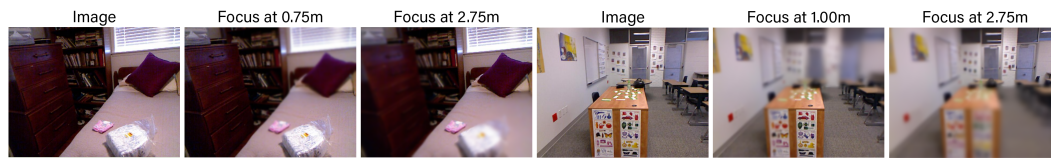
Figure 4.9 Application to synthetic defocus. We predict a depth map from a single image and use it to render a synthetically defocused image at various depths. The result is achieved by applying a bilateral filter based on the distance to the plane set in focus by the user.
