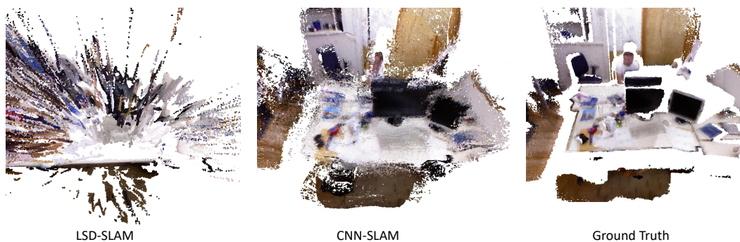
Figure 5.5 Reconstruction under pure rotational motion. We compare LSD-SLAM and CNN-SLAM reconstructions of a sequence (TUM-RGBD fr1/rpy) that consists of rotational motion.
