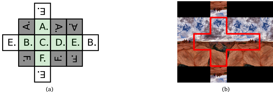
Fig. 8. Extended cutout construction scheme 8(a) and an image example 8(b). The “main”, not-extended cutout is highlighted in light green on 8(a) and in red on 8(b). A filled cutout consists of all the shaded cube faces in 8(a).
