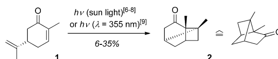
Scheme 1. The conversion of carvone ( 1 ) into carvonecamphor ( 2 ) representing the first intramolecular [2+2] photocycloaddition reaction of a cyclic enone. [6–9]
