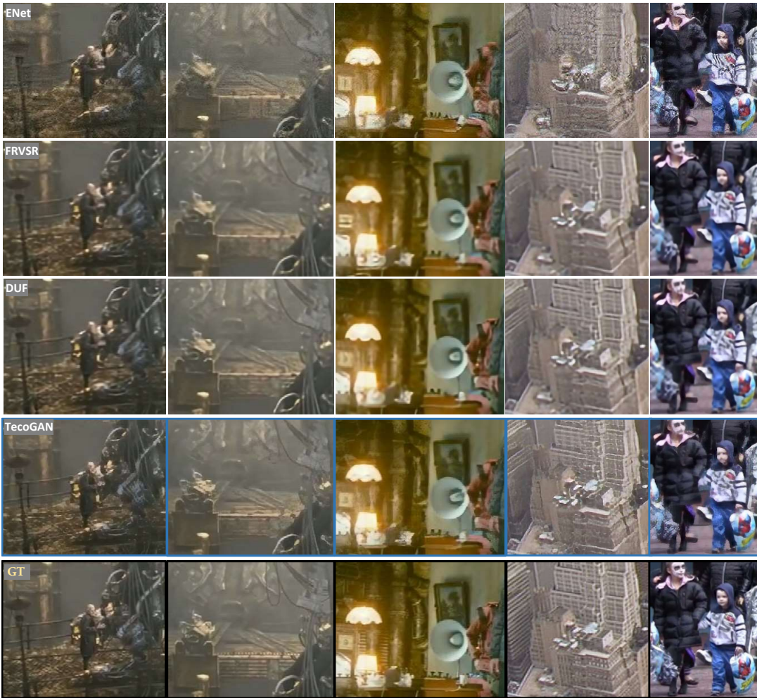
Figure 5.8: Detail views of the VSR results of ToS scenes (first three columns) and Vid4 scenes (last two columns) generated with methods from top to bottom: ENet, FRVSR, DUF, TecoGAN, and the ground truth.
