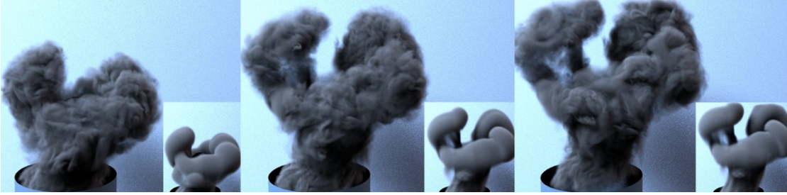
Figure 4.10: Our method applied to the flow around a cylindrical obstacle. The resolution of the underlying simulation is only 76 \times 64 \times 64 .
