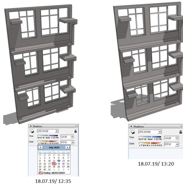
Figure 44: The overshadowing design feature of the precast concrete façade panel.
