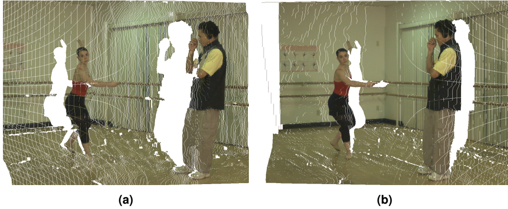
Figure 2.3.: Two examples of how the forward mapping strategy leads to tiny holes which can be seen all over the warped images (a) and (b). In contrast to the large holes which stem from the disocclusion, these are sampling artifacts due to rounding to the nearest discrete pixel location.
