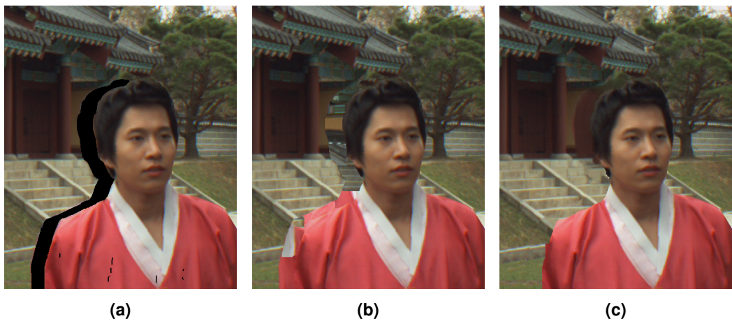
Figure 4.10.: This comparison shows how incorporating the information of the depth map can significantly improve the inpainting result of a CSH-based inpainting step. Image (a) shows the input image with the disocclusion, Image (b) shows how the result looks when using CSH without any depth information and (c) shows the result when guiding the inpainting step with the depth information. Image (b) shows areas where foreground content has been filled into the disocclusion, leading to an unnatural result.
