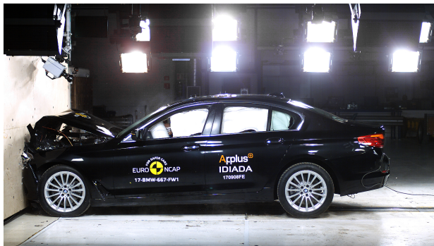
(a) Euro NCAP hardware crash test [3].
