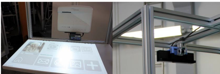
Fig. 17 User interface and Kinect sensor in the PI 2 U-MiniArc
