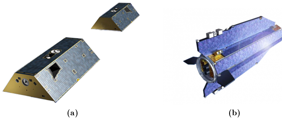
Figure 1.3.: Dedicated gravity satellite missions: (a) GRACE, observing the changing distance between the satellites. Image Credit: NASA/JPL; (b) GOCE, measuring Earth's static gravity field and ocean at the highest accuracy. Image Credit: Airbus/ESA
