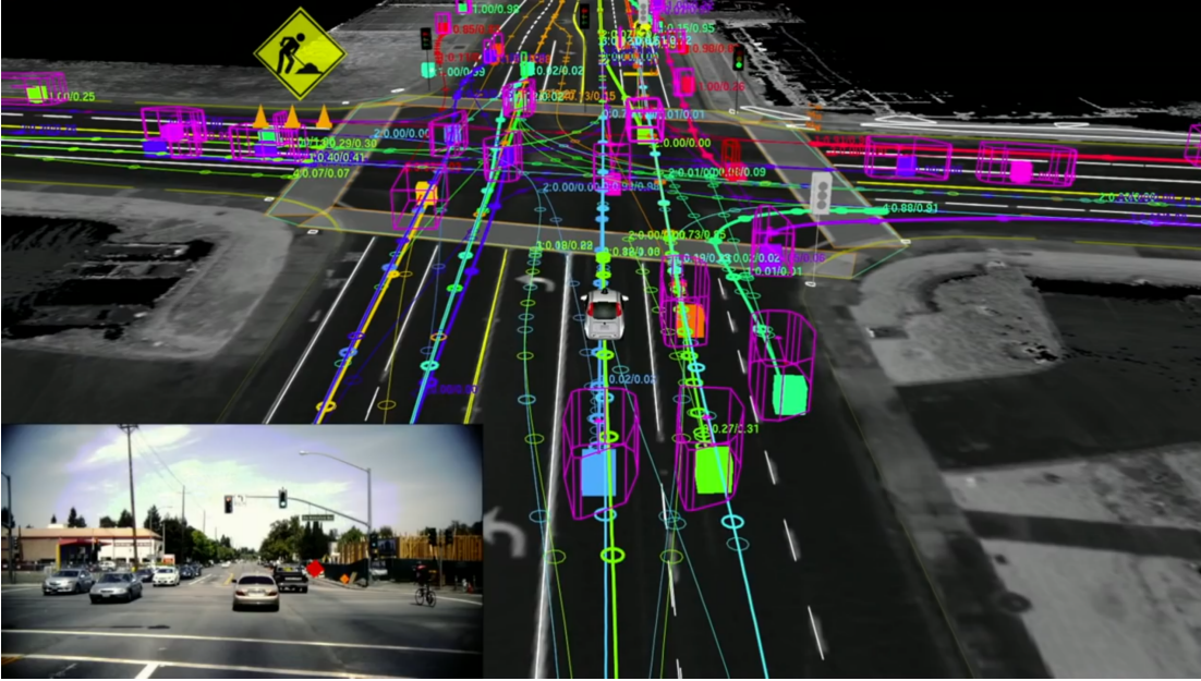
Figure 1.1. Possible prediction hypotheses anticipated by a Google self-driving car. Graphic taken from [144]. © Google 2015
