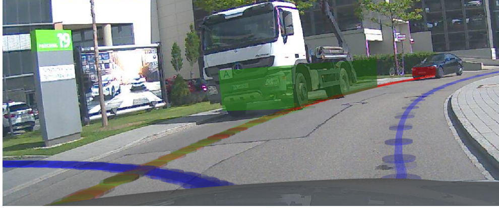
Figure 6.5. Camera view of measurement vehicle with detected objects and predicted trajectories while yielding to oncoming traffic in order to turn left into a parking lot. Previously published in [166]. © IEEE 2018
