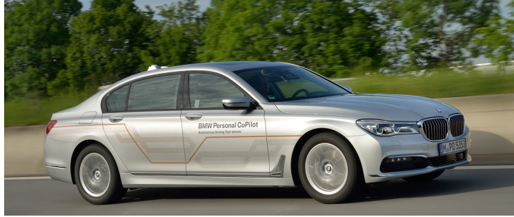
Figure 6.2. Autonomous test vehicle used to record data of surrounding traffic participants and the ego-vehicle. The vehicle is equipped with GPS/INS-based localization, as well as lidar- and radar-based object detection. © BMW Group
