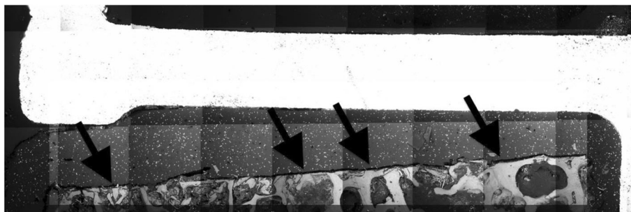
Fig. 8 SEM image, an extended area without cement penetration in area 1. Arrows, examples of how high bone density prevents bone cement from penetrating into the interspaces of the trabecular bone and thus prevents a mechanical interlocking
