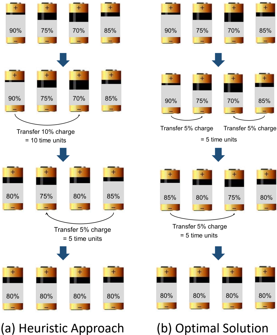
Figure 1.7: Optimal cell balancing vs existing heuristics. The heuristic takes 15 time units for cell balancing while the optimal approach takes only 10 time units. The heuristic selects non-neighbor charge transfer pairs of cells more often than the optimal approach, however, transferring charge over a larger distance results in more energy dissipation. 2
