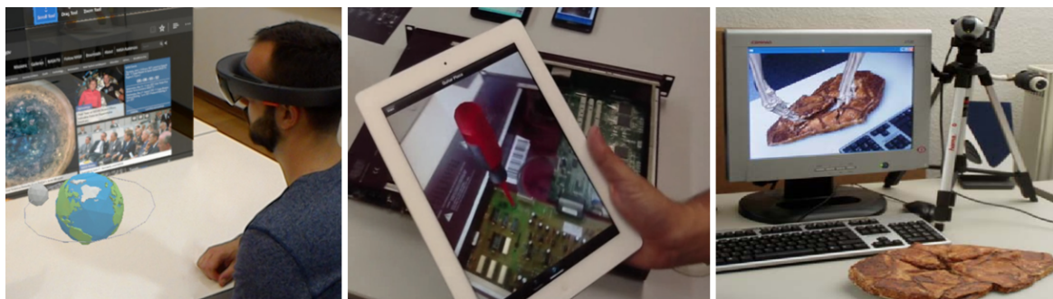
Fig. 2.4 Examples of AR displays according to categorization based on distance from the user's eye: (left) Microsoft HoloLens, a head-mounted optical see-through display [SSDM17], (middle) handheld display [GMOF13], (right) stationary display for screen-based video see-through AR [BGW + 02].
