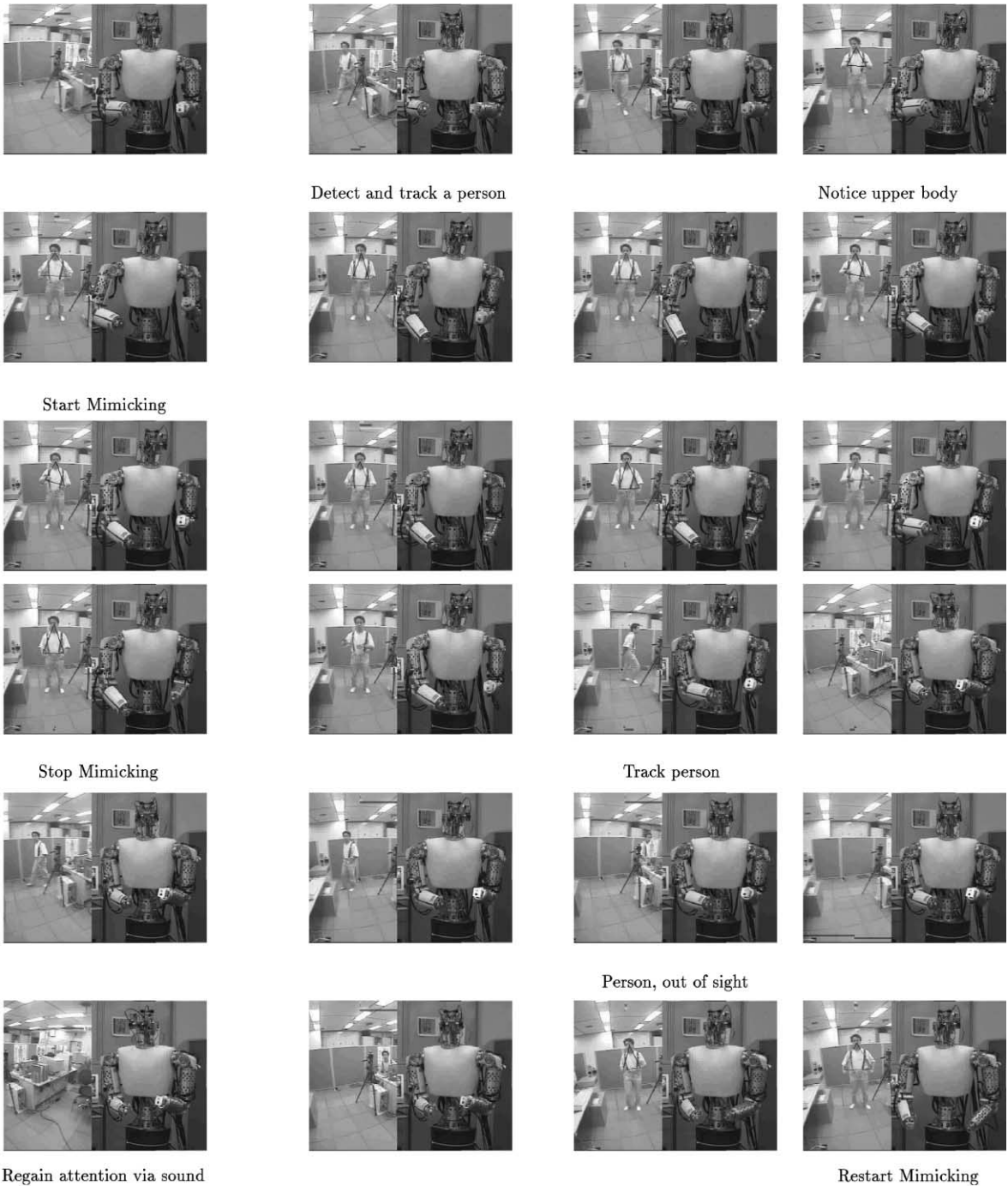
Fig. 11. Humanoid interaction: visual attention and tracking, auditory attention and tracking, mimicking of a person. This experiment shows the detection of a person, while estimating the upper body motion of the person. Detection of sound, allows our system to determine the spatial orientation of the sound source — spatial hearing. The output response of this system allows our humanoid to orientate/servo toward the person by keeping track of the person. The humanoid produces the same upper body motion as the person, thus mimicking the person. The system performs the visual processing at 30Hz in stereo, auditory sampling is performed at 44 kHz.
