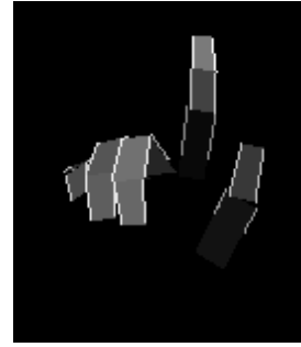
Fig. 3. Z-buffer. The depth information is displayed via the intensity of edges and areas.
