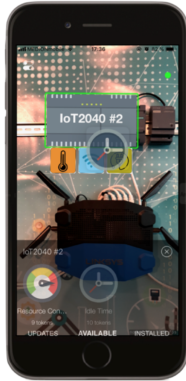
Fig. 4. AR User Interface: A technician drags and drops the app to a detected edge device. The idle time application is about to be dragged onto the edge device IOT2040 #2 . The technician must authenticate to start the installation process.
