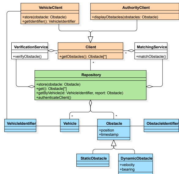
Figure 1. The Analysis object model depicts the classes derived from the requirements. The repository is the key component of the Starling system, containing entity objects like vehicles and obstacle reports. The vehicle and authority clients enable the access to obstacles stored in the repositories.
