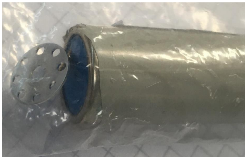
Fig. 30: 18650 cell Molicel IHR18650C with broken casing after resonance excitation. During the test the positive pole of the cell was glued to the shaker adapter, and the resonance caused the cell to break at the connection of the can and the positive cell cap [100].
